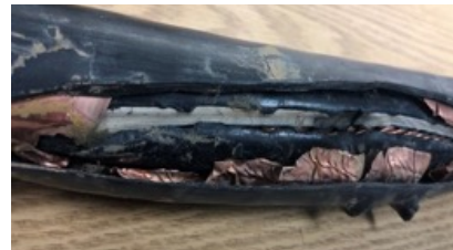
Actual examples of Excessive Pulling SWP on Cables
